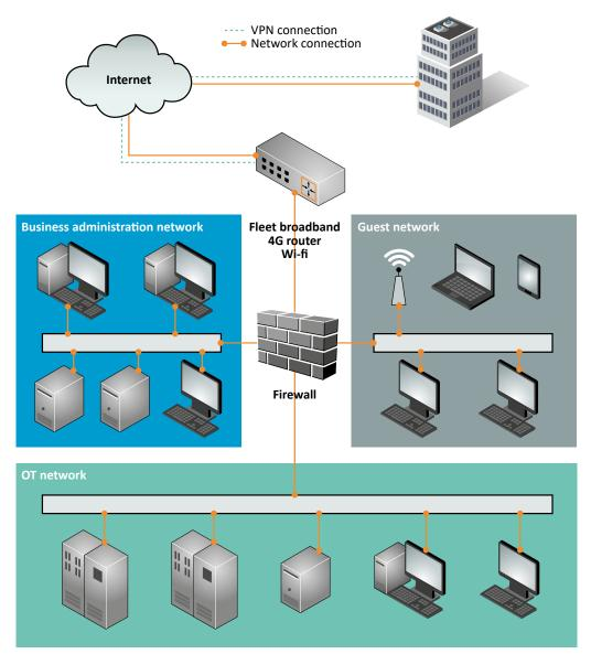
Figure 12: Example of an onboard network.
